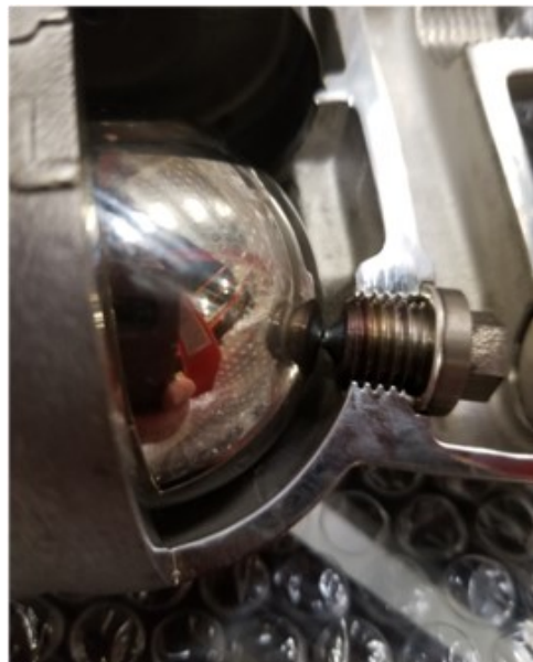
▲ Fig. 1. Free Float® steam trap has a ball float valve head and fixed orifice valve seat. The ball float enables variation of the size of the orifice opening, modulating to match flow requirements.
