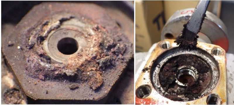
▲ Fig. 13. A steam trap may experience a lot of debris.
