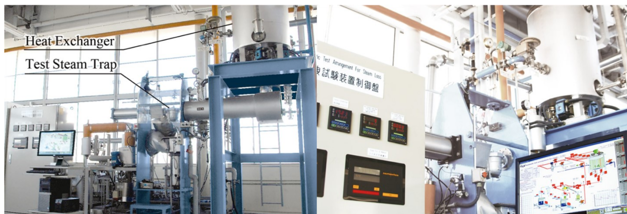
▲ Fig. 8. The test apparatus has been independently validated to comply with ASME PTC39-2005 and ISO 7841 standards.
